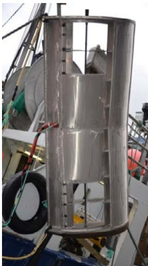
Figure 1: Manoeuvrable trawl door (left) and the effect of variable hatches on door spread at two towing speeds (right)
