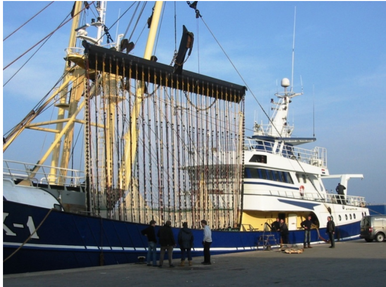
Figure 4: A pulse wing trawl with a 12 m beam
