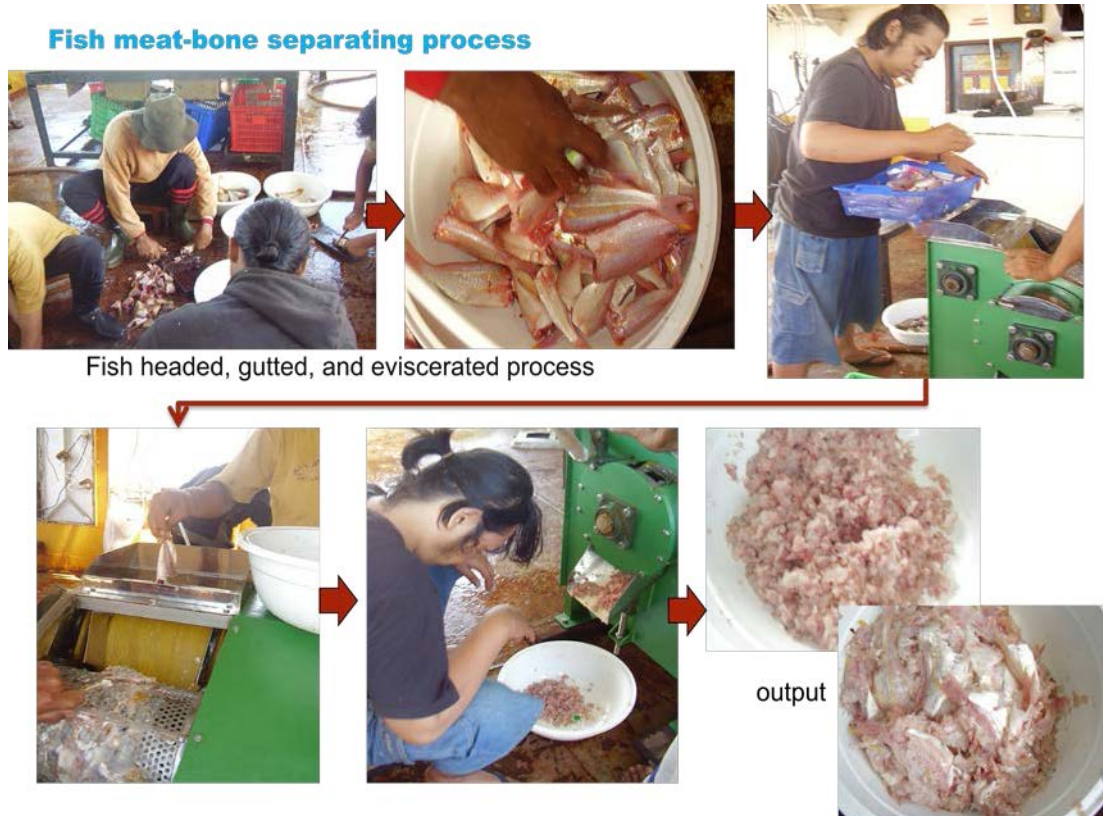
Figure 23: The fish meat-bone separating process
