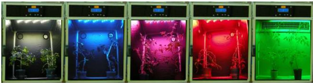
Fig. 7. Light-emitting diode (LED) chamber including broad-spectrum-white LED (BSWL, 420-680 nm), blue (460 nm), blue+red (red light supplemented with 10% blue light), Red (635 nm), and green (520 nm).
