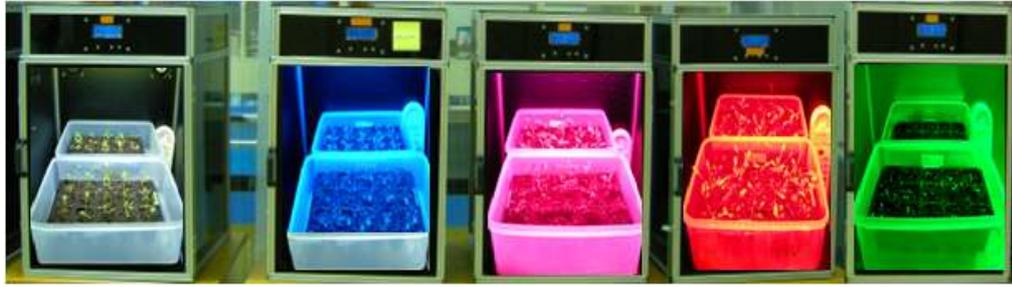
Fig. 8. Light-emitting diode (LED) chamber including broad-spectrum-white LED (BSWL, 420-680 nm), blue (460 nm), blue+red (red light supplemented with 10% blue light), Red (635 nm), and green (520 nm).
