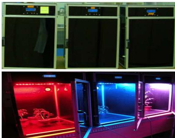
Fig. 1. Outside and inside of light-emitting diode (LED) chamber including blue LED (B, 460 nm), red LED (R, 635 nm) and green LED (G, 520 nm).
